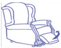
To prevent accidental damage or trapping when the leg-rest closes, each chair incorporates a sprung-loaded leg-rest. Should the leg-rest hit an obstruction on closing, it will pivot as shown to minimise pressure. The motor will only automatically cut off when the action cycle is finished. The motor may continue to function but reduced pressure will be applied to the trapped object.
